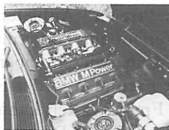
KOENIG Turbomotor 340 PS! 420 Nm, 0-100 5,2 sec., V-max. 270 km/h
