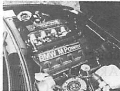
KOENIG Turbomotor 340 PS! 420 Nm, 0-100 5,2 sec., V-max. 270 km/h
