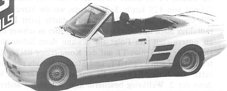
325/M 3, supersportlich, 9" × 15 – 225/50 VR 15, 11" × 15 – 345/35 VR 15, 325 – 250 PS Turbo, M 3 – 340 PS Turbo
